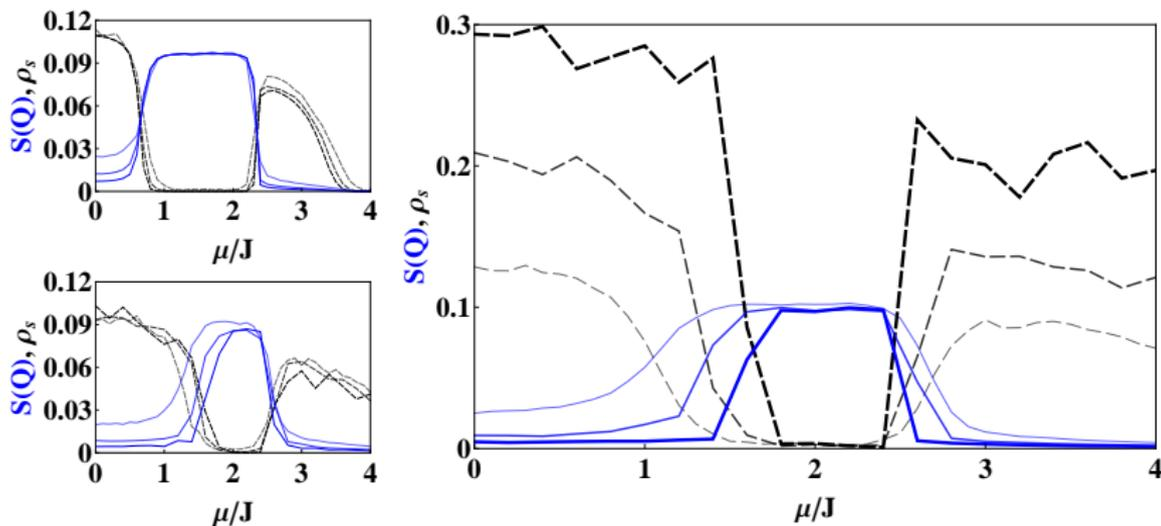
Superfluid fraction and structure factor graphs taken at 80% of the lobe ( $\theta = -0.28, \theta = -0.23, \theta = -0.15$ ) for multiple system sizes ( $L = 6, 9$  and  $12$ ). Lines get thicker and darker with system size increase.
