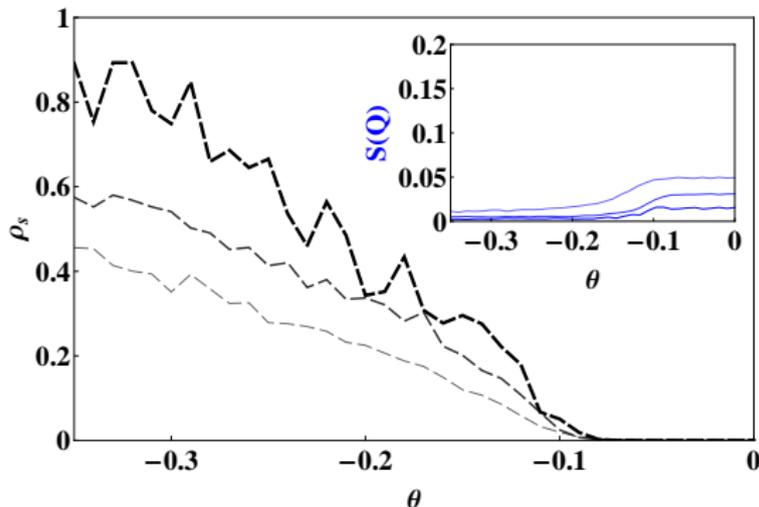
Superfluid fraction and structure factor graphs taken at  $\mu/J = 0$  for multiple system sizes ( $L = 6, 9$  and  $12$ ). Lines get thicker and darker with system size increase.
