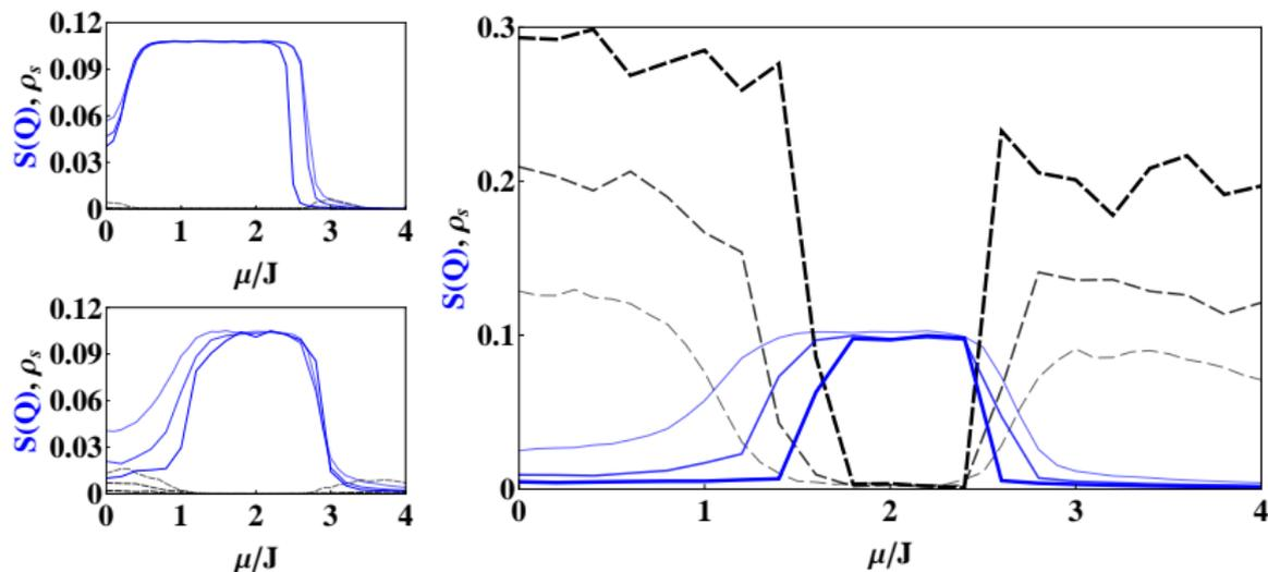
Superfluid fraction and structure factor graphs taken at  $\theta = -0.15$  for multiple system sizes ( $L = 6, 9$  and  $12$ ). Lines get thicker and darker with system size increase.
